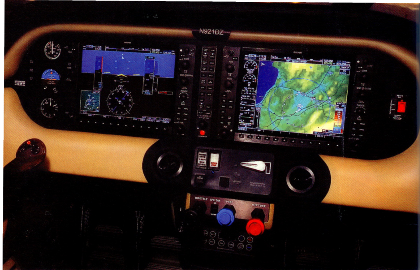
The twin 10.4-inch LCD screens of Garmin's G1000 fully integrated navigator/communicator/autopilot system bookend the vertically mounted audio control panel. Engine data is displayed on the left side of the MFD. The "go-around" button is located directly above the black throttle knob. Large air-conditioning and airflow outlets add to cabin comfort.
