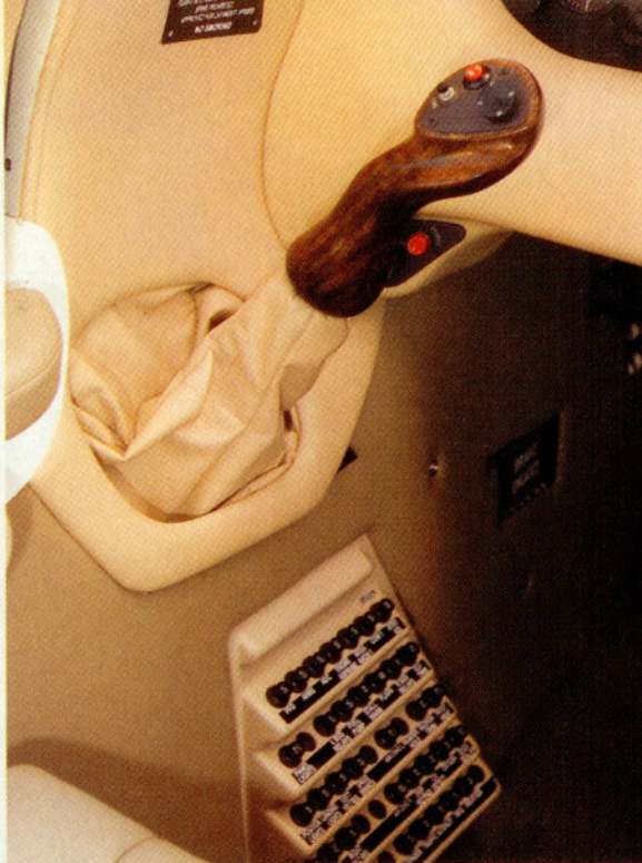
Both side-stick controls incorporate autopilot disconnect, press-to-talk, control wheel steering, and aileron and elevator trim. The black trim plate behind the yoke contains a red button for engine priming and the magneto switch. The circuit breakers nestle against the side panel.
